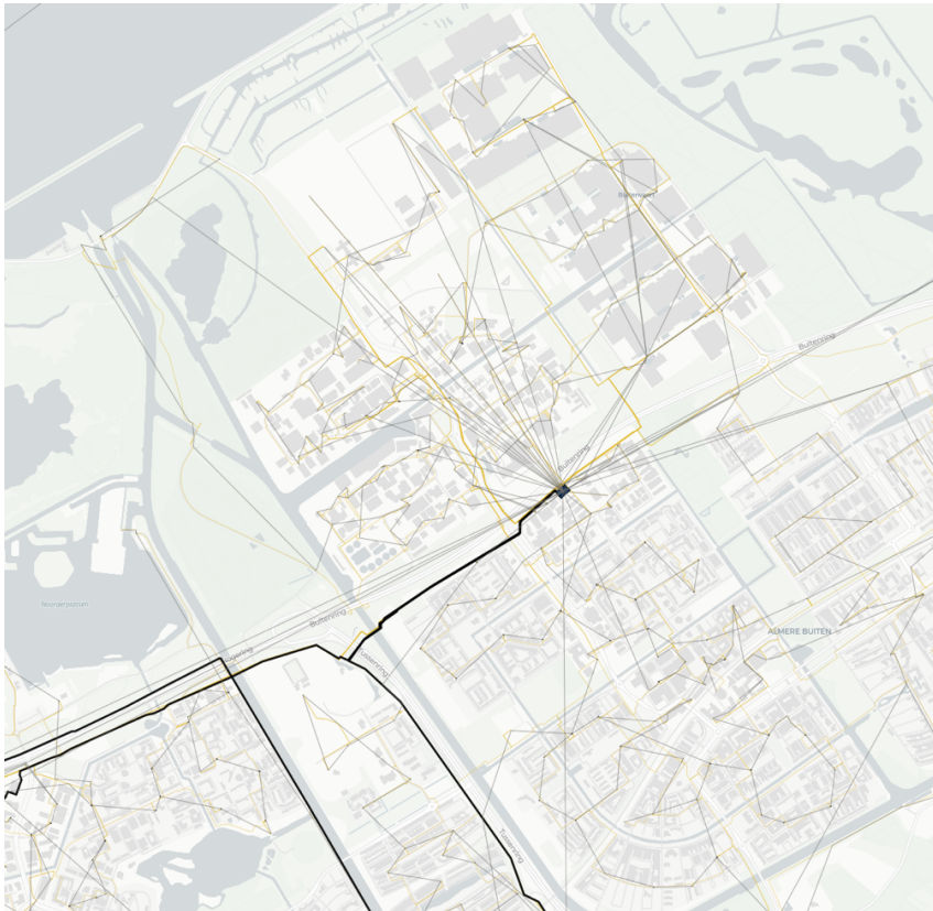
Figure 8. Illustration of the resulting network topology for a part of Almere.
