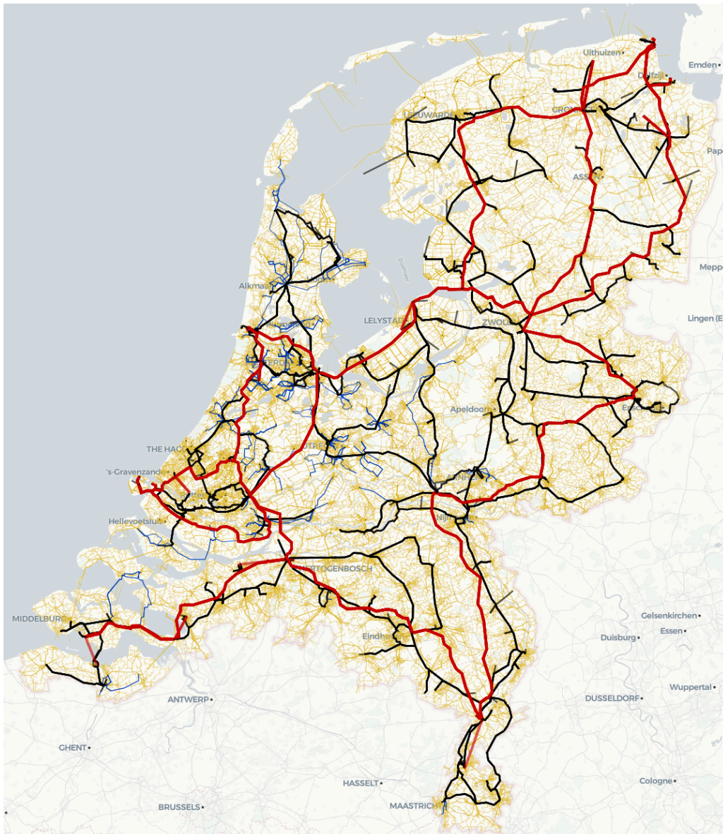
Figure 7. Cleaned location data of the EHV- (red), HV- (black), IV- (blue) en MV-nets (yellow).
